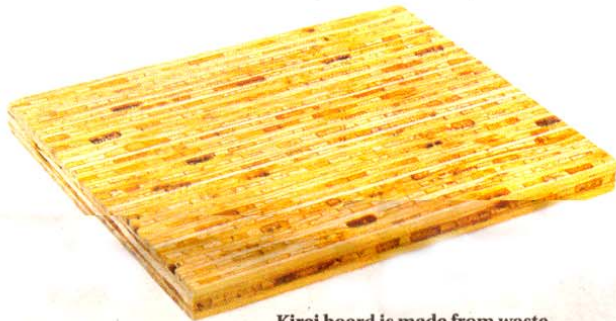
Kirei board is made from waste sorghum stalks.
