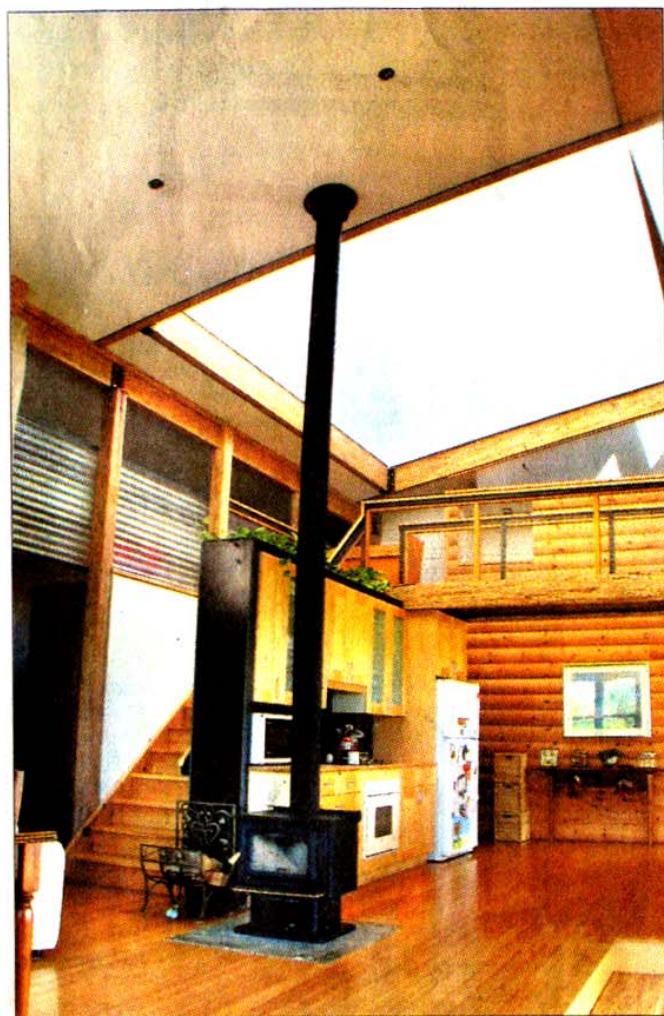
Large south-facing windows, skylights, an air-tight wood stove and energy-efficient appliances help reduce power consumption.
